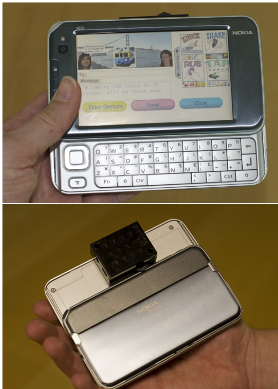
Figure 3. The SK-7 sensor box is attached to the back of the N810 to create a smooth handheld experience. The sensor box has 12 capacitive touch sensors on the outer shell.
